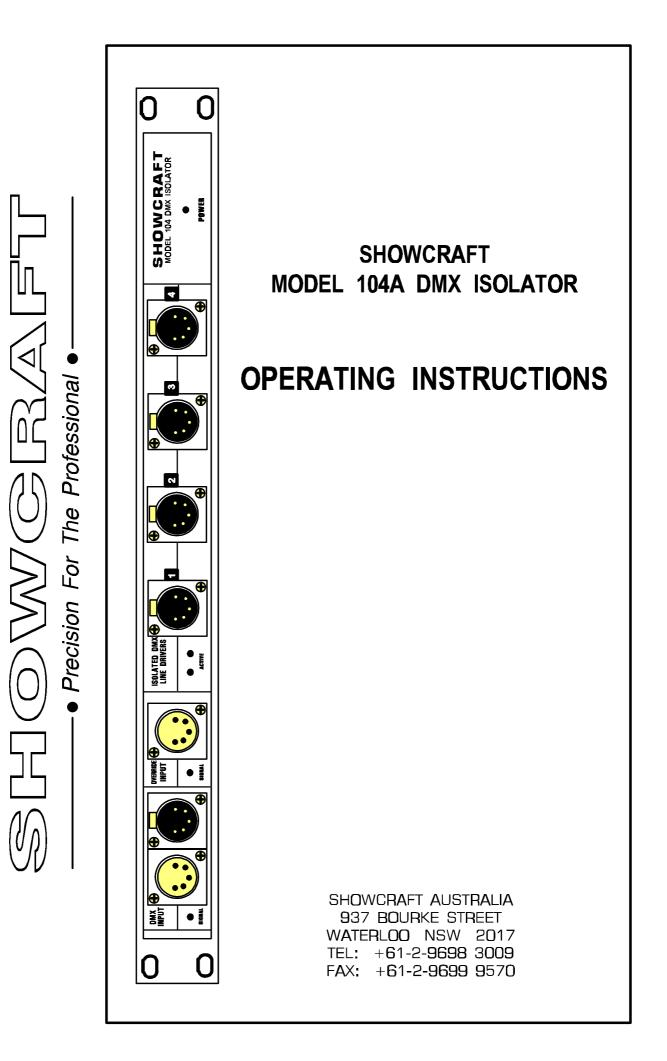
The 104 DMX isolator has four(4) output lines which can be operated from any one of two DMX input sources. The primary input is derived from the console DMX output. A second input is located on the front panel and when supplied with a DMX signal it will override any other input to the unit, this allows for a riggers control to be plugged into the system without disturbing the normal system wiring.
